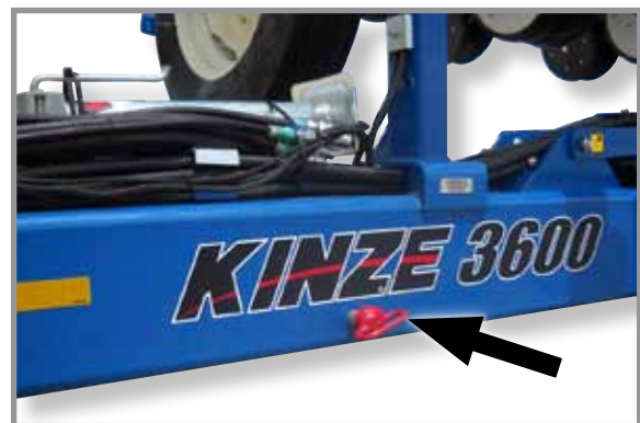
Tongue safety pin in transport position.
