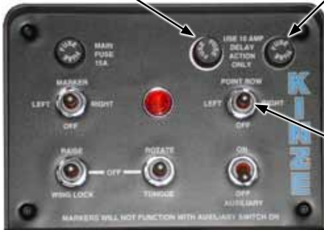
Single point row clutch control box
