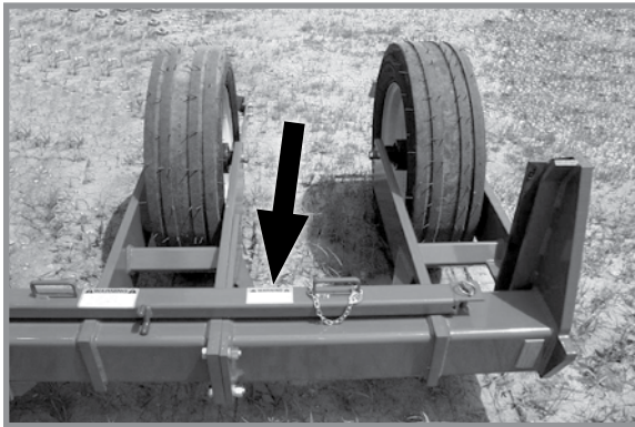
Manual safety lockup in storage position
