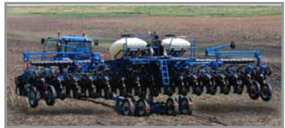
Rotate from transport to field
