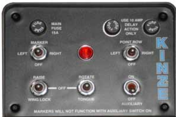
Single point row clutch control box
